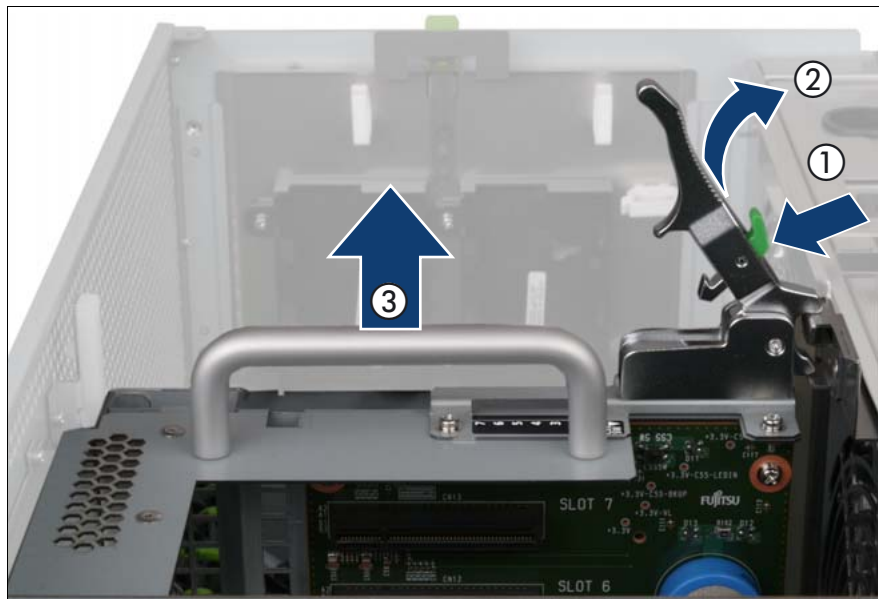
Figure 86: Removing the PCI Riser
